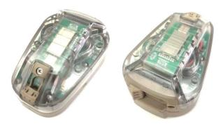
It combines high-precision UWB radio frequency positioning with light and sound warning. Primarily used in professional fields such as firefighting, security, and special police operations, it can show the real-time location of team members, solving the safety issues of firefighters in situations without 4G/5G mobile phone signals. It ensures that rescue person can be located and rescued promptly when in danger, acting as a safety protector for firefighters.
